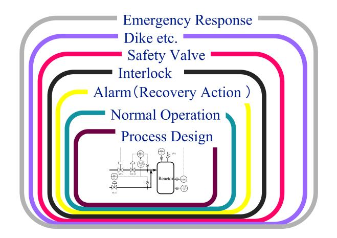
To prevent the occurrence of a system accident, several types of protective systems are installed in nuclear and chemical plants based on the concept of <u>"defence in depth"</u>.
