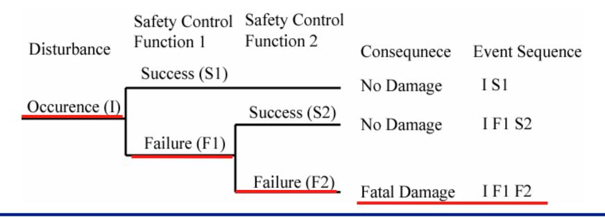
Accident sequence conditions = logical AND combination of the occurrence condition of a disturbance and failure conditions of safety control functions.
