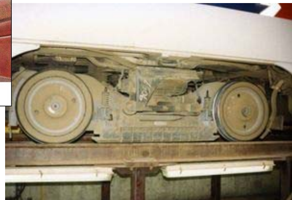
View Under Train Showing Wheelset fitted with Brake Discs. Each disc has two faces joined by vanes to assist cooling
