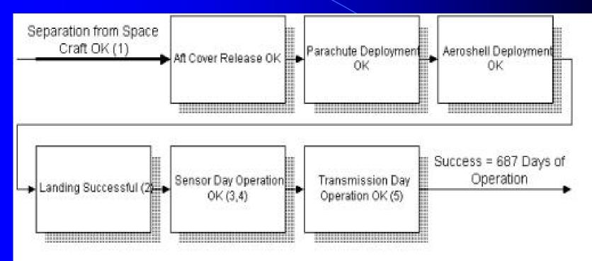
Assumes Controllers, CPU and Clock Initialized by Space Craft. No Latent Failures Owing to Launch, Cruise or Separation
