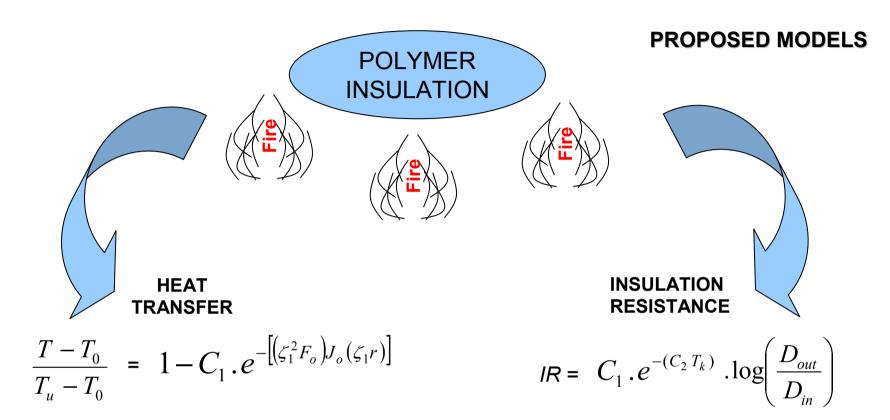
T: inner temperature of the cable at time t.To: initial temperature of the cable (t = 0).Tu: temperature in the surrounding area at time t.
