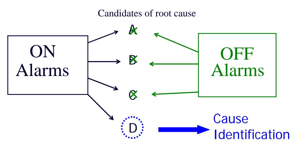
**Operators identify causes by combination of ON-Alarms and OFF-Alarms.**
